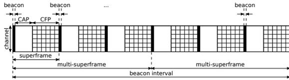
Fig. 1. Structure of an IEEE 802.15.4 DSME Beacon Interval.
