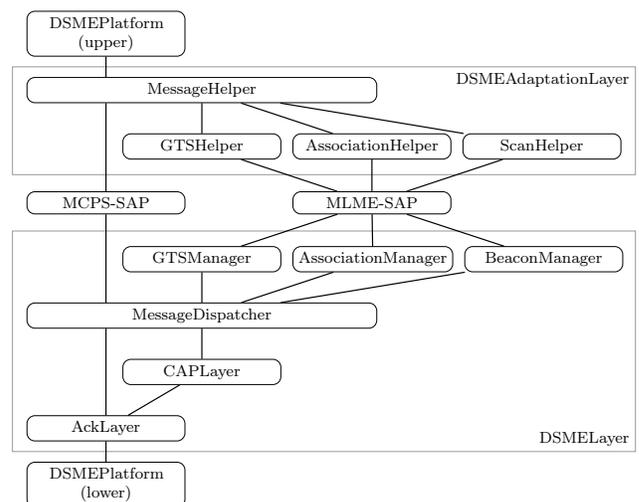
Fig. 2. Structure of the openDSME Link Layer Implementation
